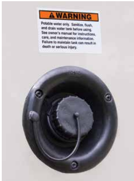
Typical fresh water gravity fill
