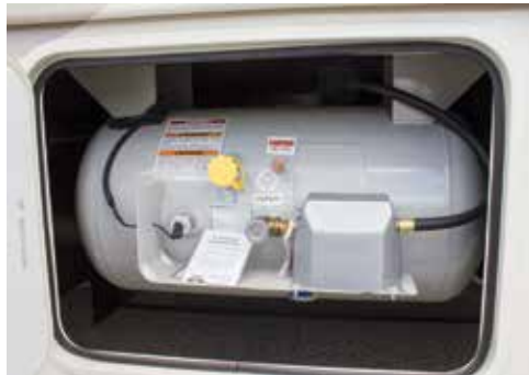
Typical propane gas tank
