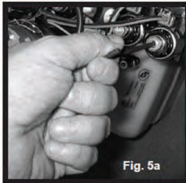
Clockwise for manual override
